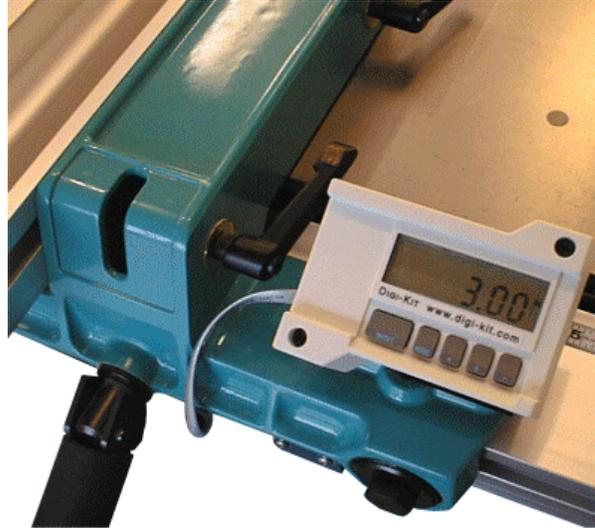
The Digi-Fence consists of three primary components, the scale which is basically the “tape”, the read head, and the display unit. The scale is screwed to the bottom of the Unifence rail and the read head slides along it sending data to the display unit via a small cable.
